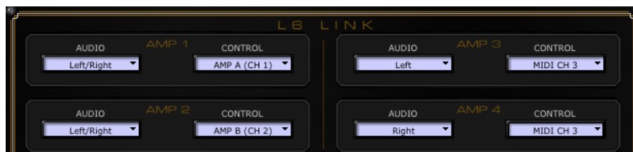
The L6 LINK Audio & Control options for up to four DT Series amplifiers
